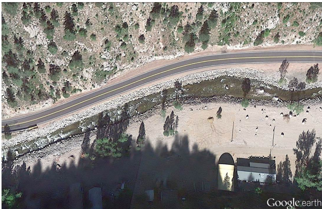
Figure 3.10. Example of post flood channel modification and bank stabilization, but with good in-channel features. (Drake).
