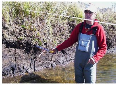
Measuring accretion on a set of bank pins
